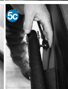
**Tip:** Use the Needle Nose Pliers when applying the Clevis Pin **19** to the Bolt Pin **1** and Sliding Pivot Arm Assembly **14 11**.
